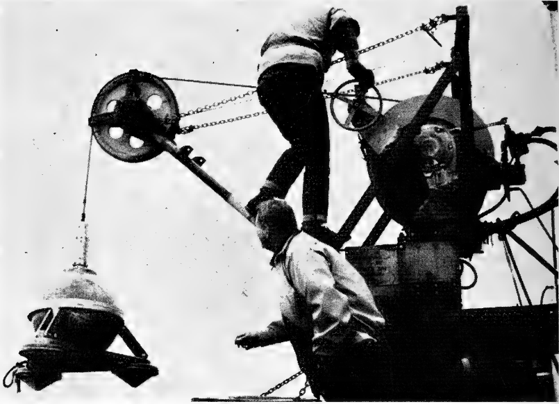
Gravity meter being lowered to the seabed to obtain measurements in establishing gravity range.
