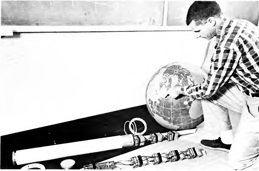
The Swallow buoy and some areas where subsurface currents have been detected with its aid.
