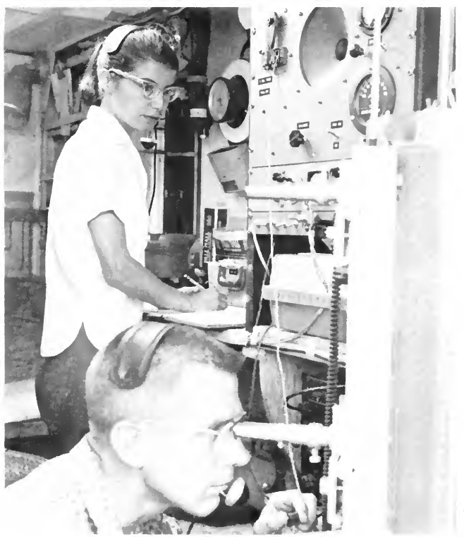
D. W. S. von Arx, assisted by Lorraine Barbour, making a gravity observation in the box-sized laboratory observa- tory mounted on the boat deck of the 'Chain'. The gravimeter employs a non- magnetic steel ball falling slowly through silicone oil of very high viscosity.
