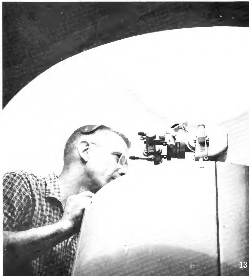
Star observations for navigation could be made by day or night with the aid of a small equatorially mounted theodolite, fixed to the head of a meridian gyrocompass.
