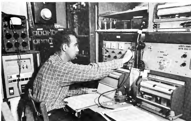
The Sea Gravimeter and part of the IBM system were built into a small air-conditioned hut in the main laboratory of the 'Chain'.
