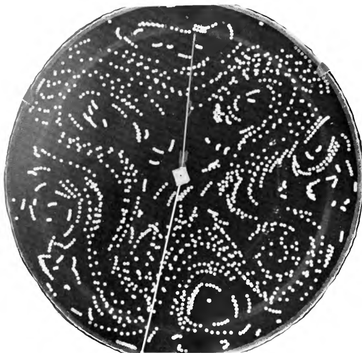
A multiple flash photograph showing the circulation in an atmospheric model. From the five images of each paper disk, floating on the water surface, the speed, acceleration, and rotation of the flow are directly determined. A four wave pattern around the tank may be readily identified.
