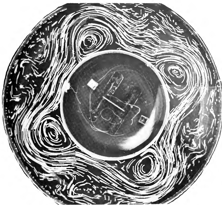
Here the flow on the water surface is indicated by streaks from paper disks during a 20 second time exposure, while the camera was rotating with the tank. By confining the flow to a channel between two vertical walls and by cooling at the central wall, four to six equally spaced regular waves may be formed. The regularity and reproducibility of these waves makes them suitable for detailed measurement.
