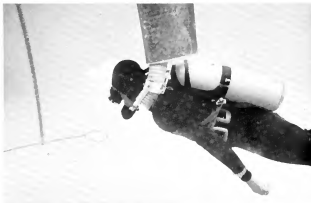
Measuring the total metabolism of a diver by way of respiratory gas exchange. The diver has to swim to keep up with the visual target at left. He receives no push from the breath collector which is attached to a turntable running along the tank.
