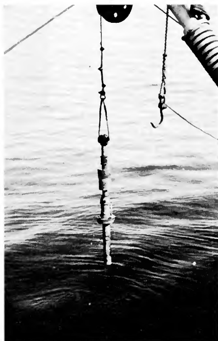
The Anderson Sampler, used to obtain sediments for bacteriological studies.
