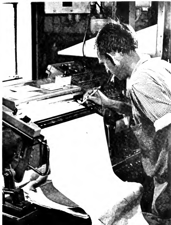
Dr. Backus checks the signals recorded on the PGR from the "pinger" on the net. Width between the lines indicate the depth of the trawl
