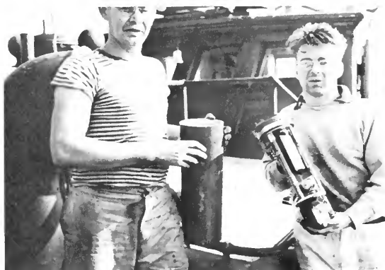
Figure 2. Ewing and Vine holding the pressure case and first deep-sea camera, on board Atlantis, 1940.
