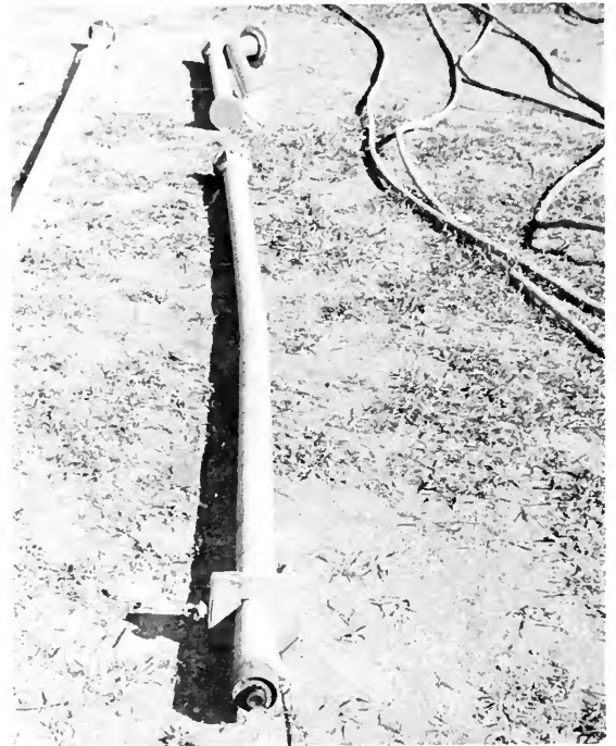
Figure 11. Underwater telescope for shallow-water work.
