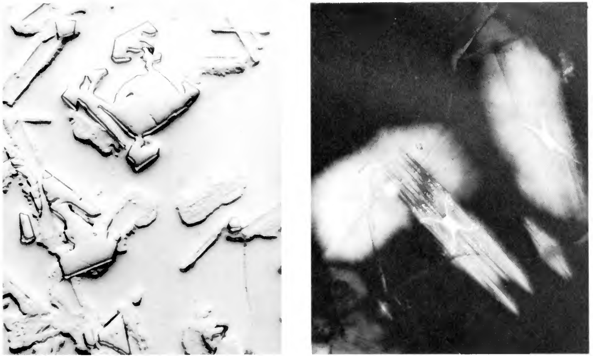
Figure 1. (Left) Reflected light interference contrast photograph of polished basalt surface, showing angular crystals of olivine and diffuse, elongated crypto-crystalline feldspar at 440x magnification. Sample is from JOIDES Site 14, South Atlantic. (Right) Transmitted polarized light photograph at 440x magnification, showing quenched olivine crystals in glass from 150-million-year-old basalt from JOIDES Site 105, northwestern Atlantic.
