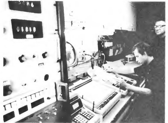
Figure 3. Inside the van aboard Lulu from which Alvin is tracked. Numbers in upper left-hand corner are travel times from Lulu or Alvin to transponders and back. This information is fed to small computer to the right, which performs a series of calculations before plotting Lulu's or Alvin's position on the x-y recorder, to its right. Author is editing raw data while monitoring the computer plot.
