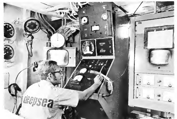
Figure 4. Oceanographer conducting a TV survey. Two monitors are used in the event one should fail. The microphone mounted on the right-hand side of the winch console is used for adding commentary to the TV tape recordings, which allow rapid annotation of important observations.
