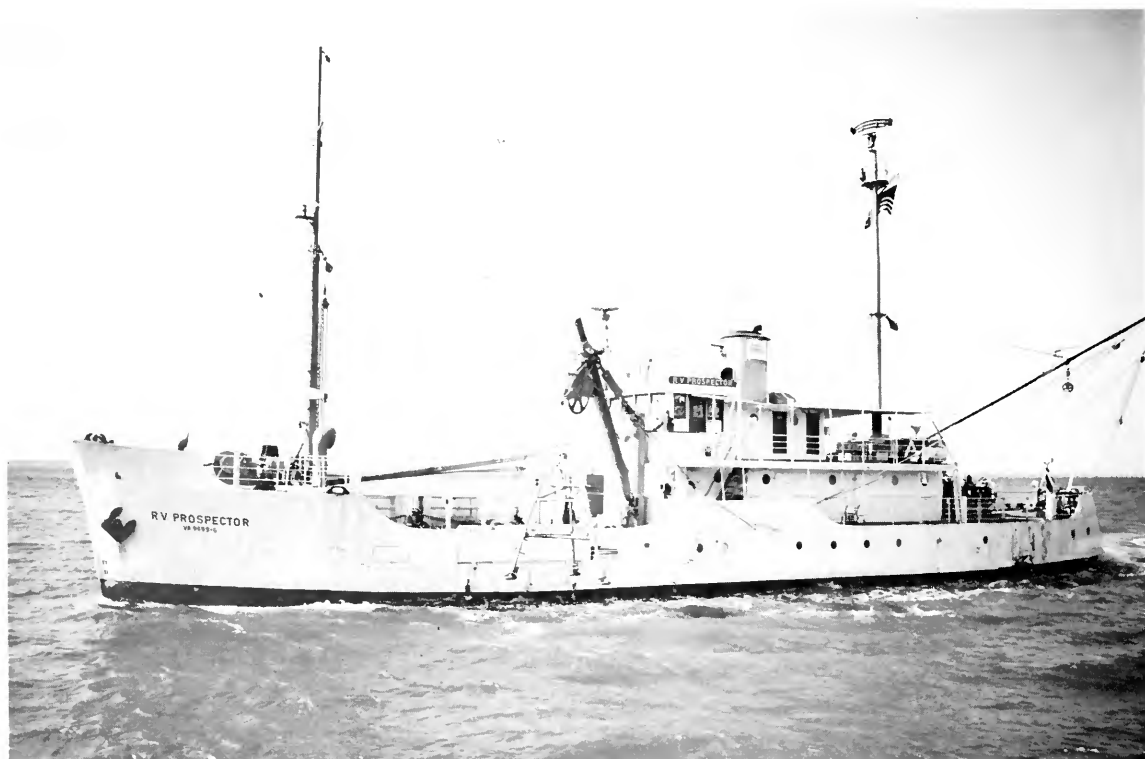
Television is deployed from Deepsea Ventures' R/V Prospector, from the main boom on the forward deck. The tripod structure provides an underwater vehicle for the electronic components and a stable platform on the sea floor (see Figure 5).
