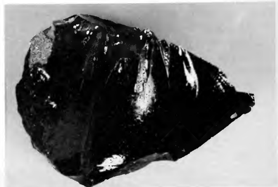
Figure 1. Silicate glass such as this would form the first "barrier" to the escape of radioactivity from the canister. The high-level wastes would actually be incorporated into the glass in a ratio of about 25 percent waste to 75 percent glass. (Courtesy ERDA)
