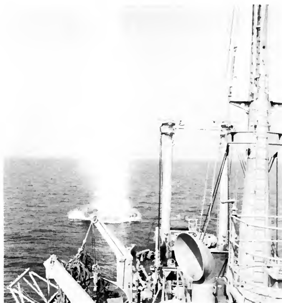
Figure 5. Beginning in 1949, explosives were used to study the spectrum of the deep scattering layers. Shots were fired at depths of less than a meter to assure sound radiation of a single pulse. The plume illustrated here was a very familiar scene at sea, when studies were underway to determine the diurnal migratory habits of small fishes in the deep ocean when responding to changing solar illumination. (Courtesy Scripps Institution of Oceanography)
