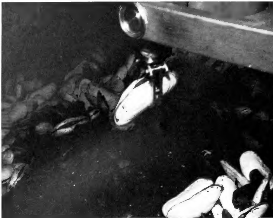
Alvin's mechanical arm picks up large clam specimen from Clambake I. Clam measured 30 centimeters (about 12 inches). (Photo by Dr. Robert Ballard)
