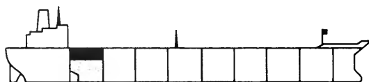
AT SEA Clean ballast for docking - Waste tank containing waste and all residues for separation
