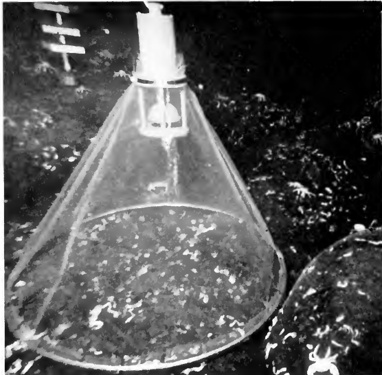
Trap to catch larvae released from the bottom. Panels in background are for studies of larval settlement. (Photo by H. L. Sanders)
