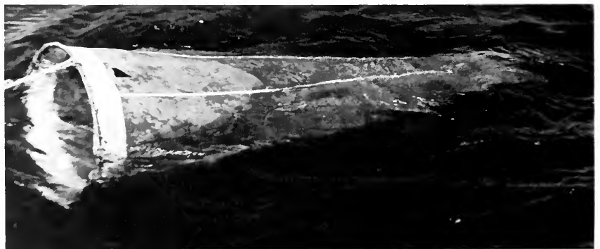
Meter net tow used to sample plankton. The distance across the face of the net is 1 meter.
