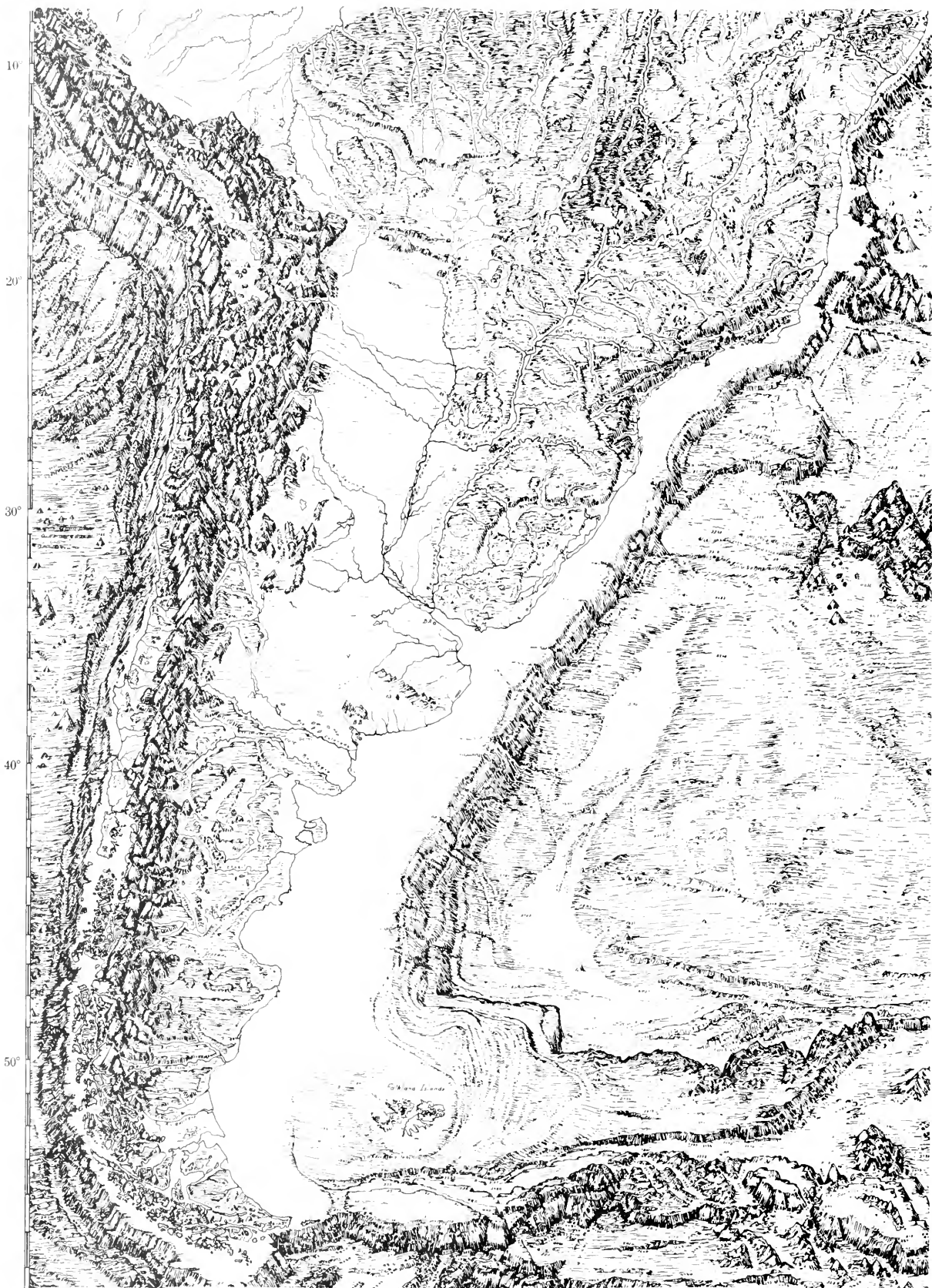
An example of the difference between Atlantic and Pacific-type margins. The eastern margin of South America is broad, with smooth expanses of sediment-covered sea floor; the western margin has a deep trench and few major sediment bodies. (From Physiographic diagram of the South Atlantic Ocean , Geological Society of America, copyright Bruce C. Heezen and Marie Tharp.)
