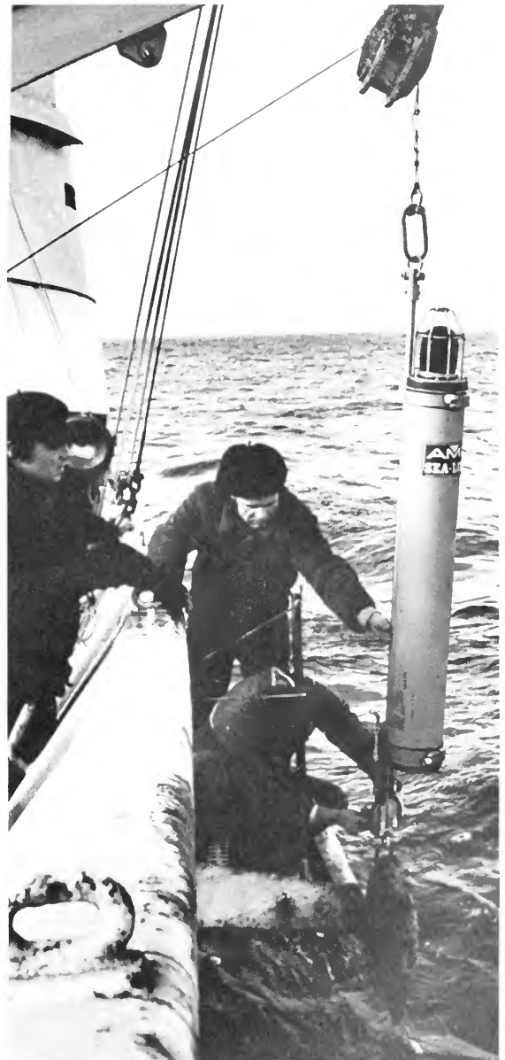
Russian scientists prepare to test an acoustic release owned by the Woods Hole Oceanographic Institution. Three Woods Hole oceanographers were aboard the Soviet research vessel for a brief cruise in 1975. A cooperative experiment was conducted, comparing Soviet and American current meters. (Photo by Robert Heinmiller — WHOI)
