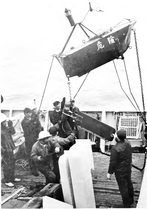
Chinese scientists prepare to deploy a surface buoy that will mark the location of moored instruments, as part of a recent joint research program involving oceanographers from China and the United States. (WHOI photo)
