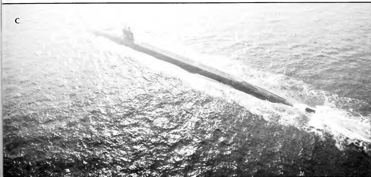
A U.S. task group (A), consisting of the carriers Kitty Hawk, Midway, and Nimitz, steams through the Arabian Sea. (B) The Navy’s Tomahawk cruise missile, launched from a submarine. (C) The USS Ohio, the first of the Navy’s new Trident submarines. Larger than any U.S. submarine before it, the vessel carries 24 Trident missiles, each with multiple warheads and a range of 4,000 nautical miles. (Photo courtesy of General Dynamics Corporation). (D) A cruise missile launched vertically from a surface ship. Turning once clear of the launcher, such missiles are aimed electronically. (Photos A, B, and D courtesy of U.S. Navy)
