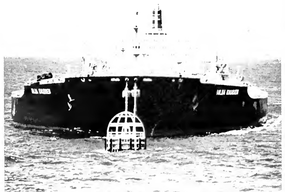
The Hilda Knudsen, a supertanker of 417,000 deadweight-tons, unloading oil at a LOOP mooring buoy. (Photo courtesy of LOOP, Inc.)
