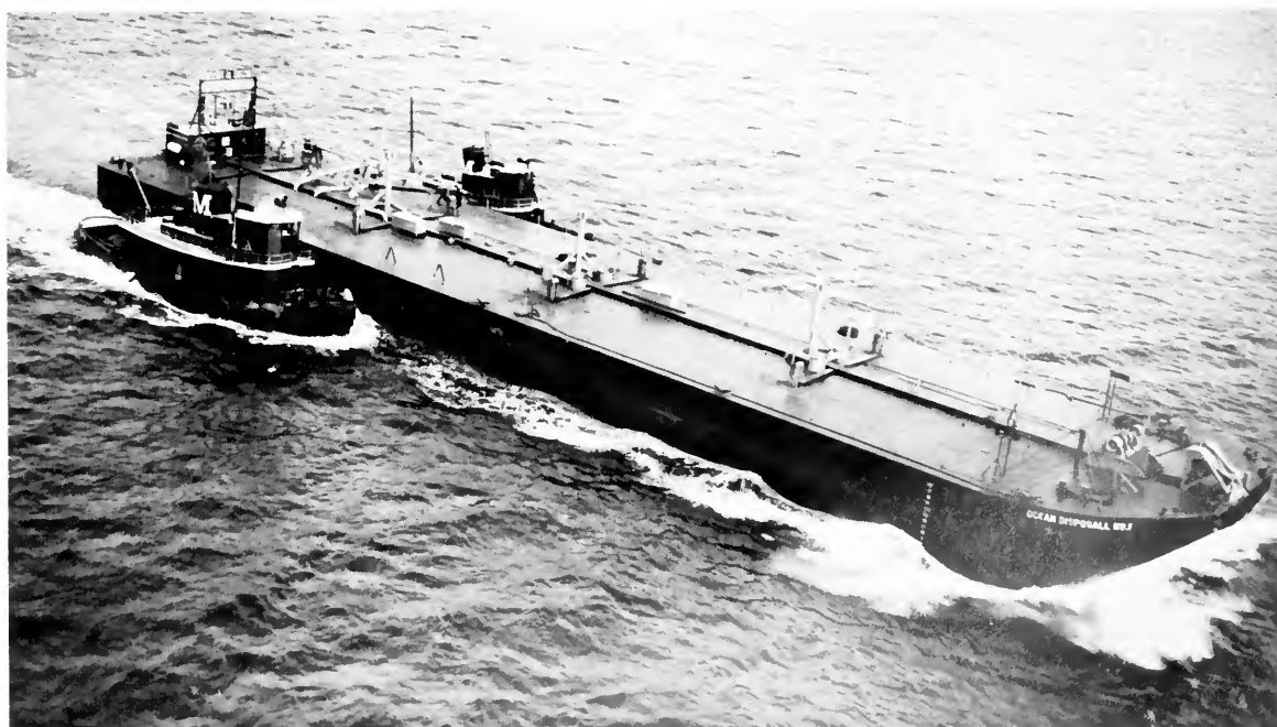
Nine sewerage authorities in the New York City area have been dumping sewage sludge into the Atlantic Ocean since the 1920s at a site 12 miles equidistant from New York and New Jersey beaches. Here a tug guides a barge full of sludge out to the site. The tug and barge keep moving during the discharge in order to disperse the waste. Some authorities use self-propelled tankers. (EPA photo)
