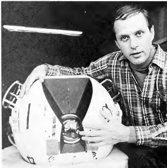
Robert D. Ballard, Associate Scientist at the Woods Hole Oceanographic Institution, with an early prototype of Jason, a remote cable vehicle equipped with a television camera for an "eye." Deployed from Argo, a towed vehicle with an array of sonar and camera systems, Jason will one day eliminate the need for a human presence on the deep seafloor (see Oceanus , Vol. 25, No. 1, p. 30). (Photo by Ira Wyman)
