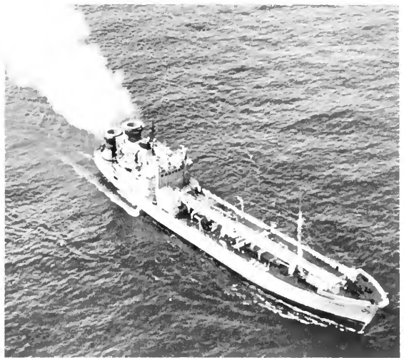
Incineration at sea. Here the Vulcanus, a specially designed disposal tanker, burns polychlorinated biphenyls (PCBs) in the Gulf of Mexico. With the incinerators set at 1,350 degrees Celsius, PCBs break down into hydrochloric acid and water, which forms a vapor that precipitates into the water behind the ship. The PCBs were drained from spent or recalled transformers and other electrical components. (Photo courtesy of Waste Management, Inc.)
