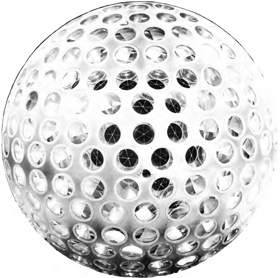
Figure 1. The Laser Geodynamic Satellite (LAGEOS) was fitted with special surfaces to reflect laser light beams from sources on the earth. Measurement of the laser transit time yields accurate information about the earth's rotation. This is one of several techniques presently used to measure length of day (lod). (Photo courtesy of NASA)
