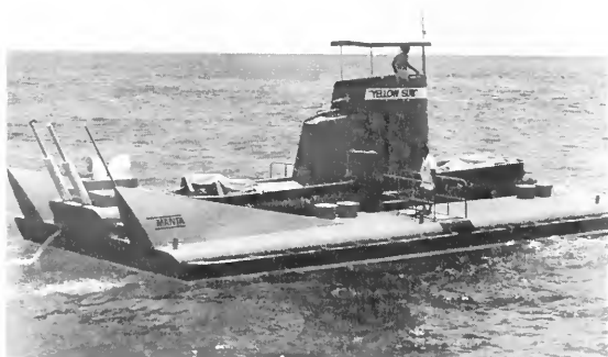
The Yellow Sub, a semi-submersible vessel that allows non-divers to explore the Great Barrier Reef of Australia. Passengers observe through underwater windows.
