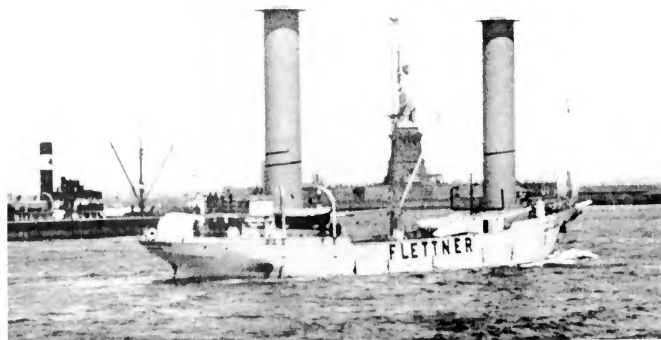
Above: The crew prepares to dock. Two diesel engines facilitate this sort of maneuvering. (Photo by Shelley Lauzon) At left: The Flettner rotor ship in New York after crossing the Atlantic. (Photo courtesy Yachting, CBS Magazines, copyright June 1926)
