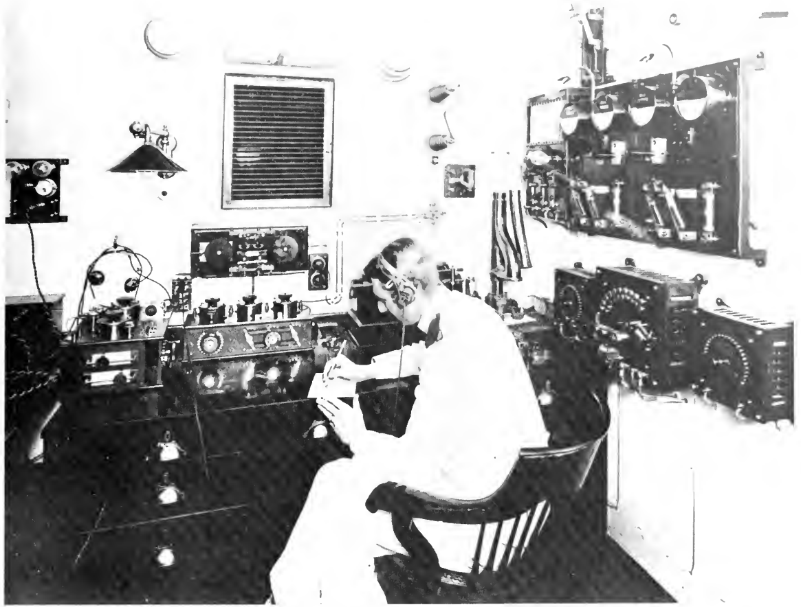
Marconi Marine 1912 installation, as fitted in the wireless room of the Titanic. At left is a valved receiver with headphones; fitted to the wall is the magnetic detector and, beneath this, the Marconi/Franklin multiple tuner; partly obscured by the head of the operator is the 10 inch induction coil spark transmitter. On wall at right are the controls of the power generator, housed in the adjoining cabin. (Photo courtesy The Marconi Company, Ltd.)
