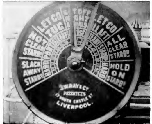
The starboard telegraph on a docking bridge of the Olympic . A similar telegraph from the Titanic can be seen on page 28. (Photo courtesy of Blackhawk Films)
