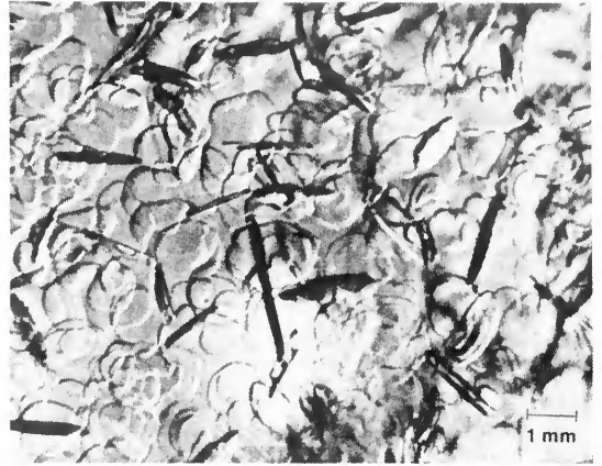
Frazil ice, showing spine-like crystals. (From Weeks and Ackley, 1982. The growth, structure, and properties of sea ice . CREEL Monograph No. 82-1)
