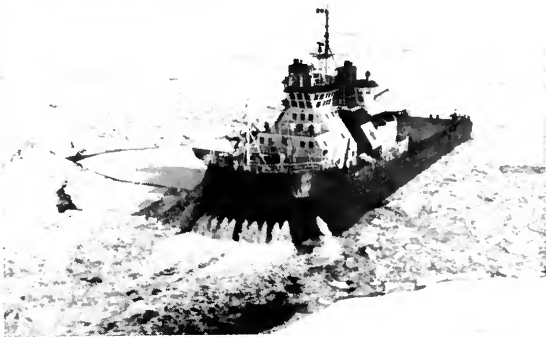
The Robert Lemeur has water jets to lubricate the hull and improve icebreaking efficiency. This ship is used primarily for support of oil drilling operations in the Canadian Arctic. (Photo courtesy of Canadian Marine Drilling)
