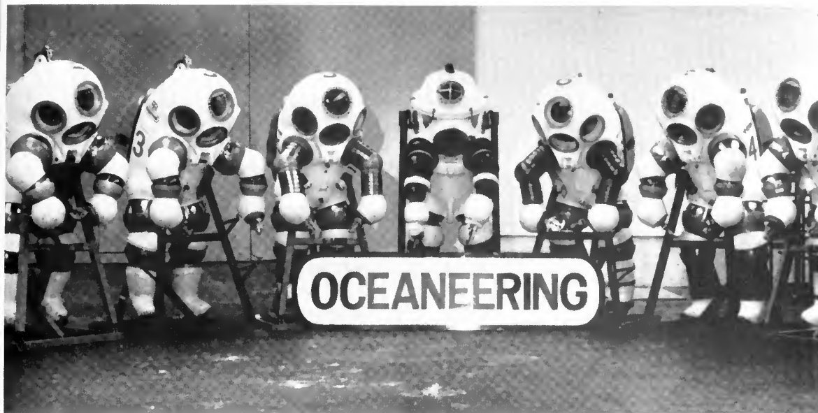
A fleet of 15 Jim suits have been built for operation worldwide, mostly in support of offshore oil operations. The operator supplies muscle power, but Jim relies on a tether for communication and deployment. (Photo by Graham Hawkes)
