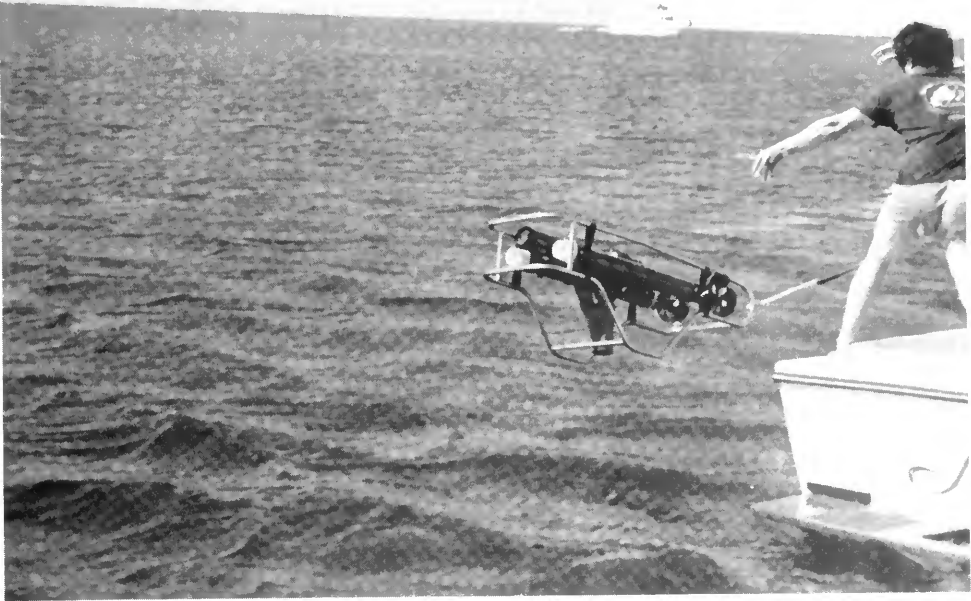
Easy to deploy, Phantom vehicles and other small, portable ROVs can readily be handled by one or two people working from a small boat. (Photo by Sylvia Earle)
