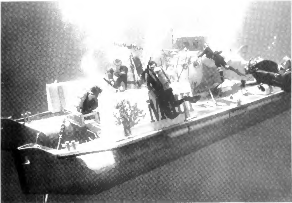
The LRT, with the submersibles Jim and Star II aboard, submerged at a dive site off Hawaii. The completely submersible launch-and-retrieval platform, or LRT, operated by the University of Hawaii avoids difficulties sometimes encountered when using conventional techniques in less-than-optimum weather and wave conditions. (Photo by Sylvia Earle)
