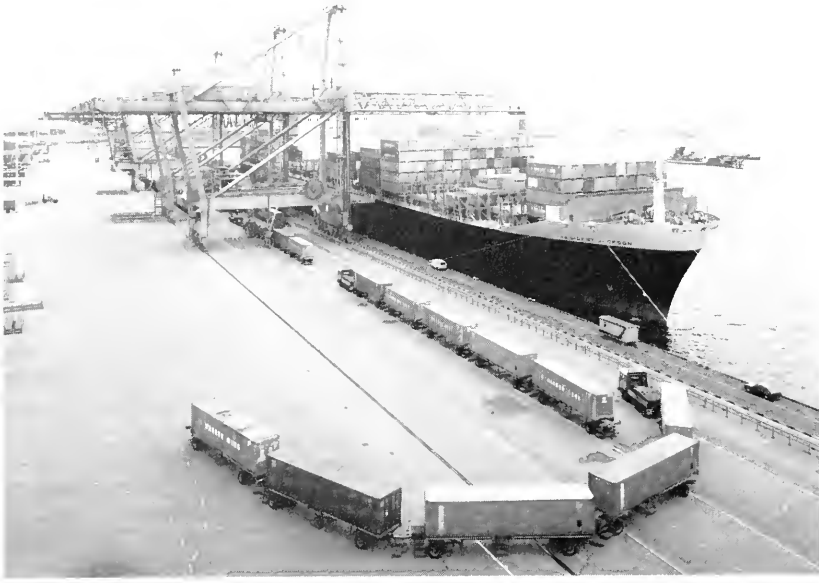
The cars of the multi-trailer system employed at ECT's Delta Terminal have computer-controlled steering, allowing each car to follow precisely the path of the car preceding it. (Photo © by Photo Sea Sky Martin)
