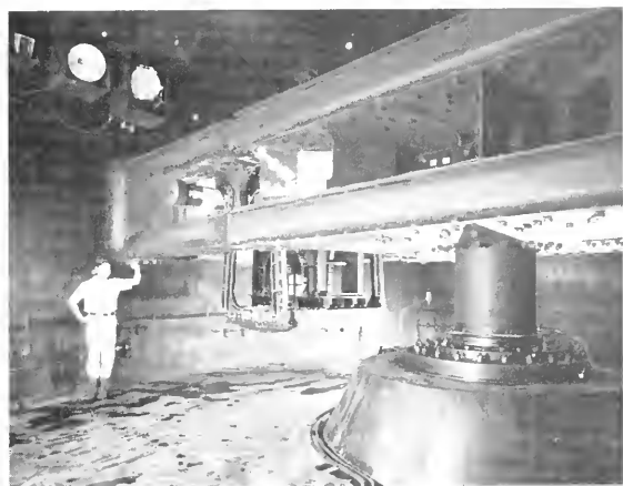
The Geotechnical Centrifuge at the Ports and Harbors Research Institute, Yokosuka, Japan.
