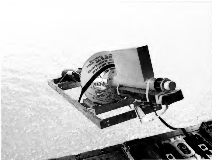
NAVOCEANO deployed more than 250 satellite-linked drifting buoys during 1990. This buoy, which measures the wind speed and direction, wave height, temperature of the air and water, and barometric pressure, is being deployed from an Air National Guard C-130 in the western Pacific Ocean.
