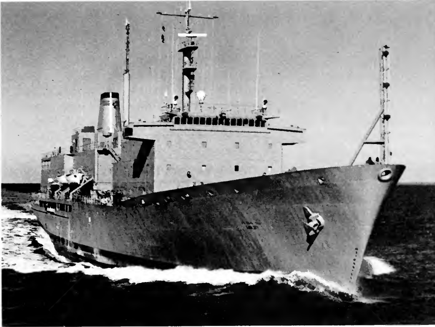
USNS Maury is a geophysical survey ship used for data collection by the Naval Oceanographic Office.
