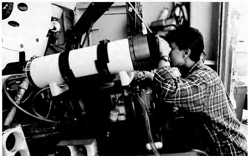
Sheri White checks the alignment of the ALISS filter array during a fall 1997 cruise.
