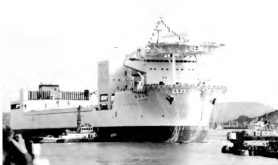
A NEW DRILL SHIP —The Integrated Ocean Drilling Program's drill ship Chikyu ("Earth" in Japanese) is launched in Japan, in 2002. The 57,500-ton, 210-meter (689-foot)-long ship will be capable of drilling 7 kilometers (4.35 miles) below the seafloor—sufficient to reach the mantle. Its derrick was installed in September 2003 and after sea trials, Chikyu should be ready by late 2006.
