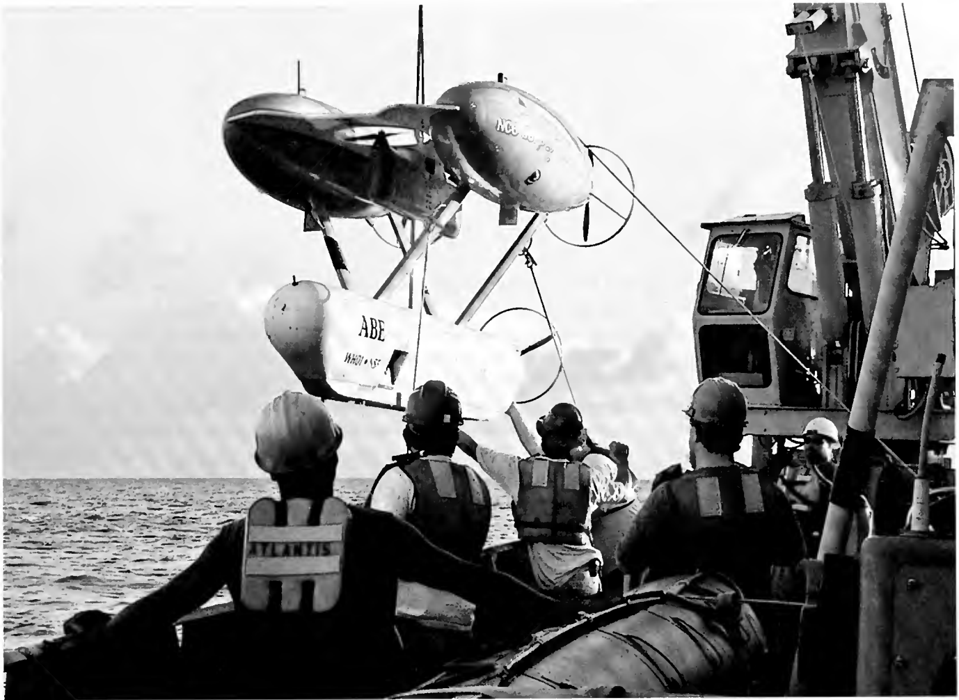
THE AUTONOMOUS BENTHIC EXPLORER (ABE)— Developed by Al Bradley, Dana Yoerger, and colleagues at WHOI, ABE can maintain a stable ride and constant altitude over changing seafloor topography. It can make detailed seafloor maps and collect high-resolution magnetic data.
