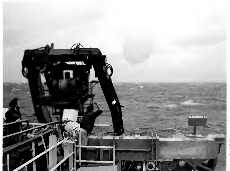
▲ Atmospheric scientist Jim Edson launches a radiosonde—an instrumented weather balloon—from R/V Atlantis .
