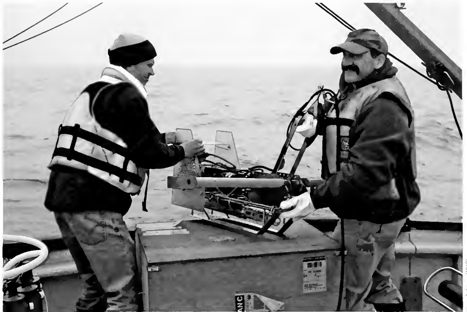
▲ Steve Okkenen from the University of Alaska, Fairbanks, and Phil Alatalo from Woods Hole Oceanographic Institution deploy the Acrobat, an instrument towed by the boat to measure water temperature, salinity, and fluorescence. The research team deployed a variety of instruments to examine the oceanic conditions that bring copepods to coastal waters.
