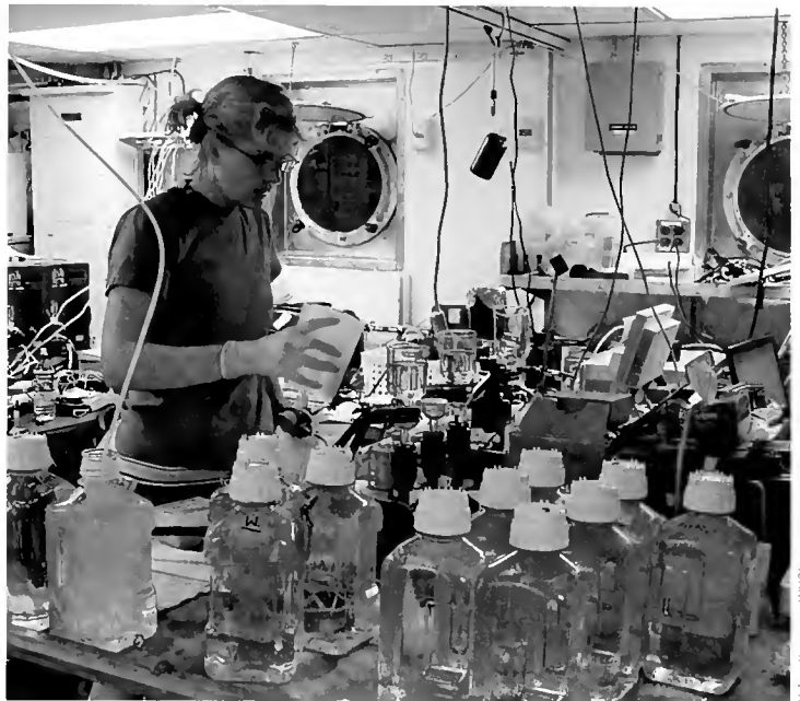
▲ Sarah Bender, a Rutgers University researcher, processes water samples in the laboratory on R/V Oceanus . She is measuring how nutrients affect the abundance of microscopic plants in the eddy.
