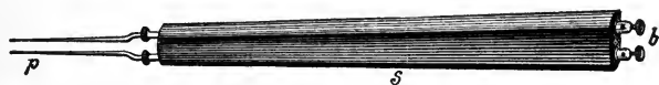
Fig. 29.—Stimulating (catheter) electrodes for nerves: b , Binding posts for attachment of wires from the secondary coil; s , insulating sheath of hard rubber; p , platinum points laid upon the nerve.
