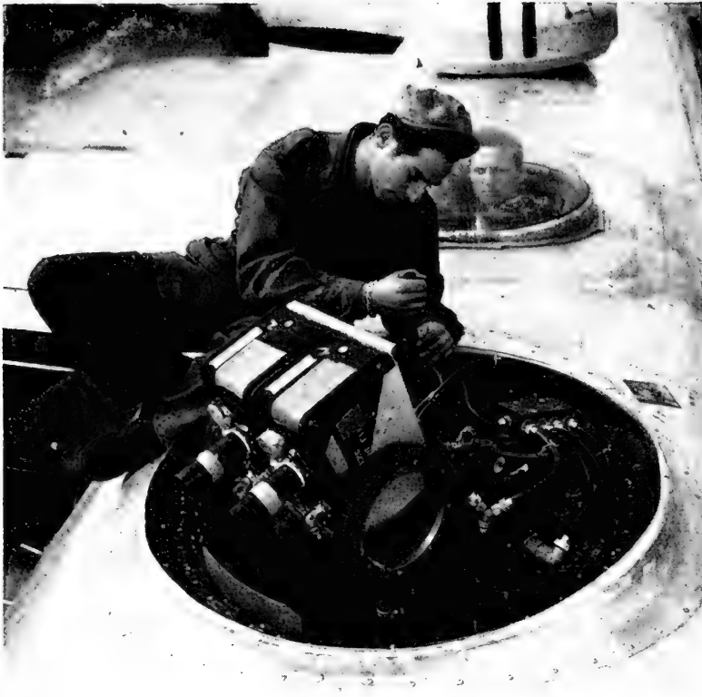
PREFACE TO PRECISION. On a Boeing F-13 plane altered for use as a photographic ship two motion picture cameras are installed in one of the plane's gun turrets. These cameras were controlled from the top fire control blister shown in the background by the same sighting and firing mechanisms normally used with the plane's machine guns. Shown here at Roswell Field, New Mexico, are Corporal Harold Johnson, outside the plane, making adjustments on the cameras, while Sergeant Henry R. Zarnoski mans the controls in the top fire control blister. In the background, can be seen another turret, slotted cover in place, housing a similar motion picture camera installation.
