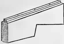
Top end of Rafter.
