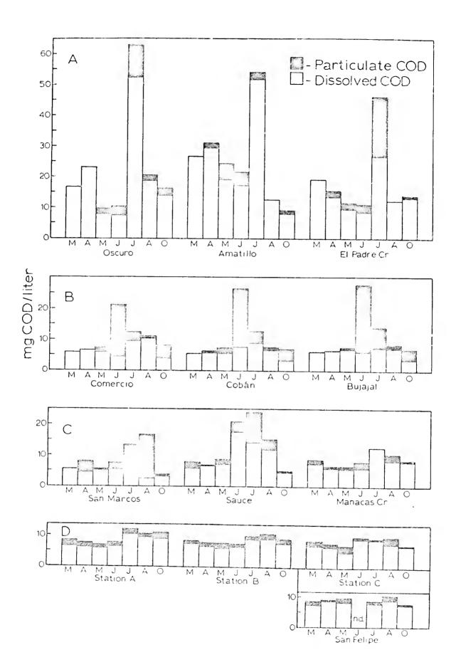
COD values. The slightly higner COD concentrations at 3 m (Appendix, Table F-1) in March and April may represent real differences (relative to surface) since the 3-m water was anaerobic. Inorganic reducing substances could have contributed to the COD at 3-m depth since the test docs not distinguish between organic and inorganic reducing compounds.
