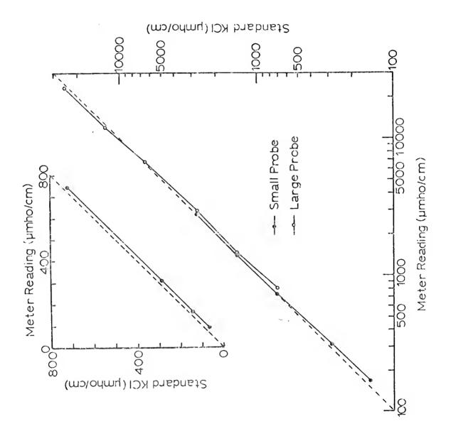
required less precision since detecting differences in the salinity gradients was more important than acquiring absolute values. Nevertheless, the calibration curve is in close agreement with the standard KC1 solutions (Figure 5).
