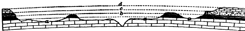
FIG. 19.—Diagram showing the successive variations of fertility in the soils of central Kentucky during the downward movement of the rocks. a, a, a , parts of the present surface enriched by decay of limestones; b , next preceding stage, when soils rested on Devonian shales and were moderately fertile; c , yet earlier stage, when soils were formed on millstone grit and were very lean; d , earliest stage when soils rested on the coal measures, and were moderately fertile. For simplicity of illustration several stages of variation are omitted.
