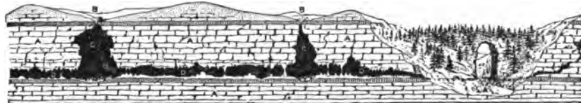
FIG. 5.—Diagram showing action of soil water in excavating caverns. a a , layers of limestone, easily dissolved in soil water; b b , sink holes by which the soil water enters the cave; c c , vertical shafts or domes; d d , horizontal galleries. The arch in the middle entrance is a natural bridge or remnant of a large cave.
