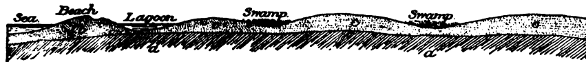
FIG. 23.—Diagrammatic section from seashore to interior of district recently elevated above the sea level. a a, bed rocks; b, beach deposits and dunes; c c, marine sands with gently rolling surface.
