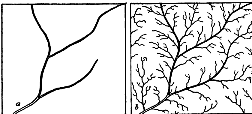
FIG. 4.—Map showing comparative development of stream beds in a district when it is forested and when the wood is removed. a , forested state; b , deforested state.
