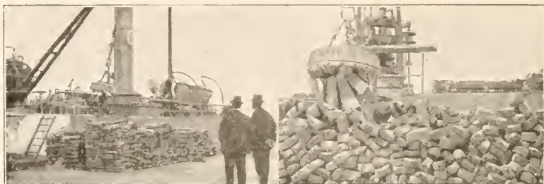
TAKING ON A CARGO OF PIG IRON BY MEANS OF ELECTRIC LIFTING MAGNETS. NOTE HOW THE PIGS FLY TO THE MAGNET
