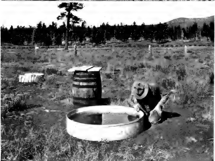
Figure 29. At the Fort Valley Forest Experiment Station, Coconino National Forest, Arizona. A typical meteorological station. Note the shelter which contains thermometers and also the electrically equipped instruments to record the direction and velocity of the wind.
