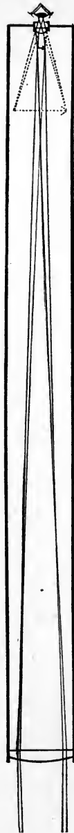
FIG. 148.—Diagram of telescope. The nearly parallel rays of light from the distant object are focused so as to form an image near the eyepiece, which acts as a magnifier to enlarge it. In opera glasses an extra lens is added to make the image appear right side up.
