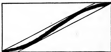
FIG. 42.—Diagram of the end of the block from which a propeller is cut.
