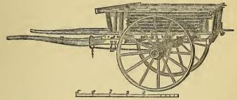
moveable spars or poles are stowed on the outside of the cart, which may, in a few minutes, be unpacked and placed upright round the frame-work, adapting it to the carriage of bulky articles of forage, such as hay or straw. Some of these spars, again, are fitted to be placed as ridgepoles on the top of the uprights, for the purpose of supporting a canopy for the protection
