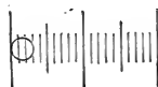
FIG. 40.—Ordinary form of eye-piece micrometer, with a human blood corpuscle, magnified 300 diam., seen through it.
