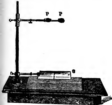
FIG. 280.—Hering's Apparatus for Simultaneous Contrast with Binocular Vision by two Doubly Refractive Prisms, P, P. G. Glass to avoid reflection.
