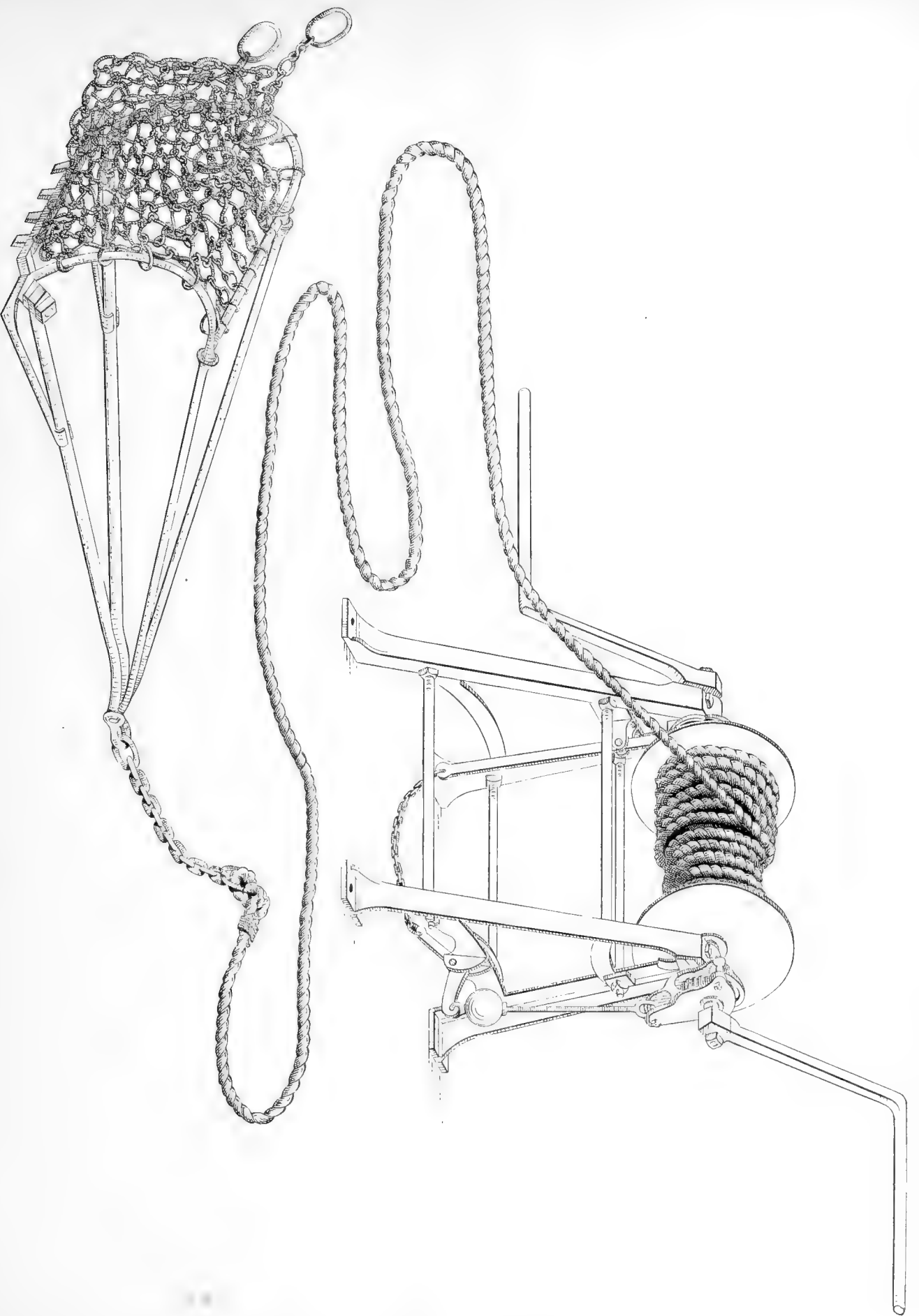
CHESAPEAKE OYSTER-DREDGE WITH WINDLASS. [From specimen in U. S. National Museum.]
