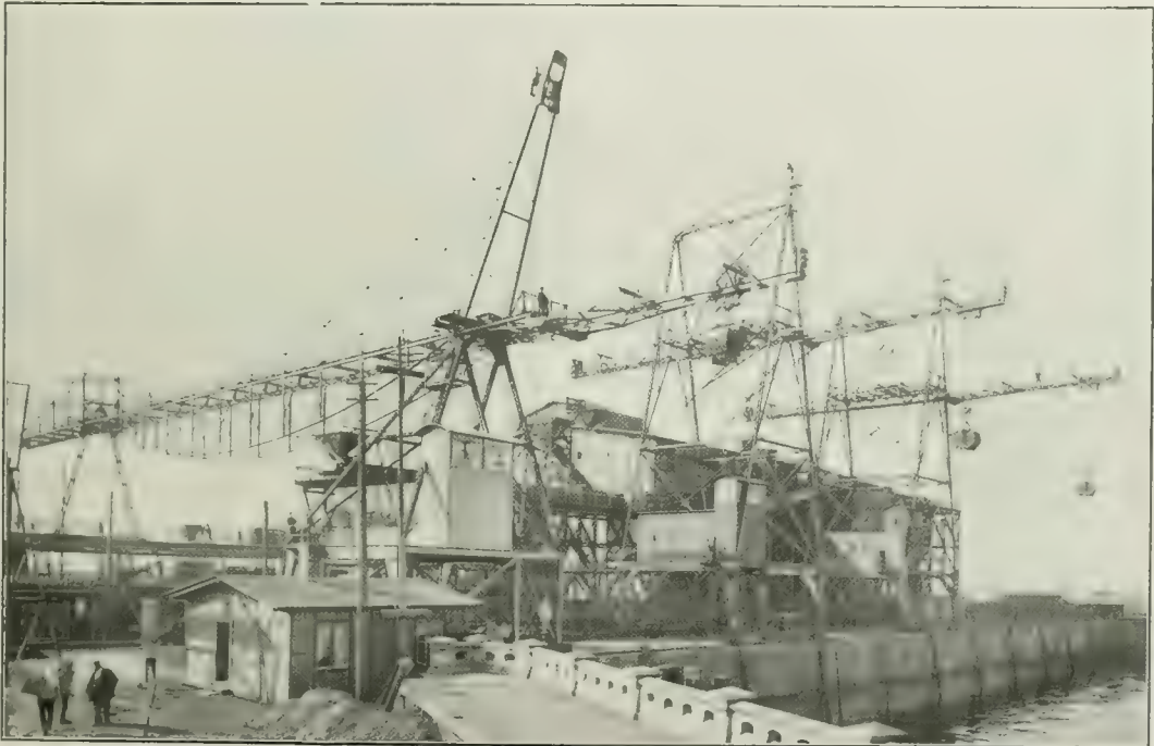
Hoisting and Conveying Plant, erected for the Norddeutsche Kohlen & Coakswerke a.g. Hamburg. These Three Cranes unload 1,500 Tons Cargoes in Ten Hours.
