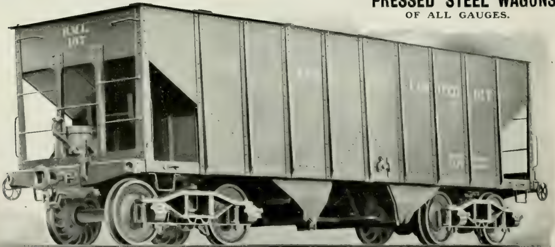
30-Ton Self-Clearing Coal Hopper Wagon, as used in South Africa.
