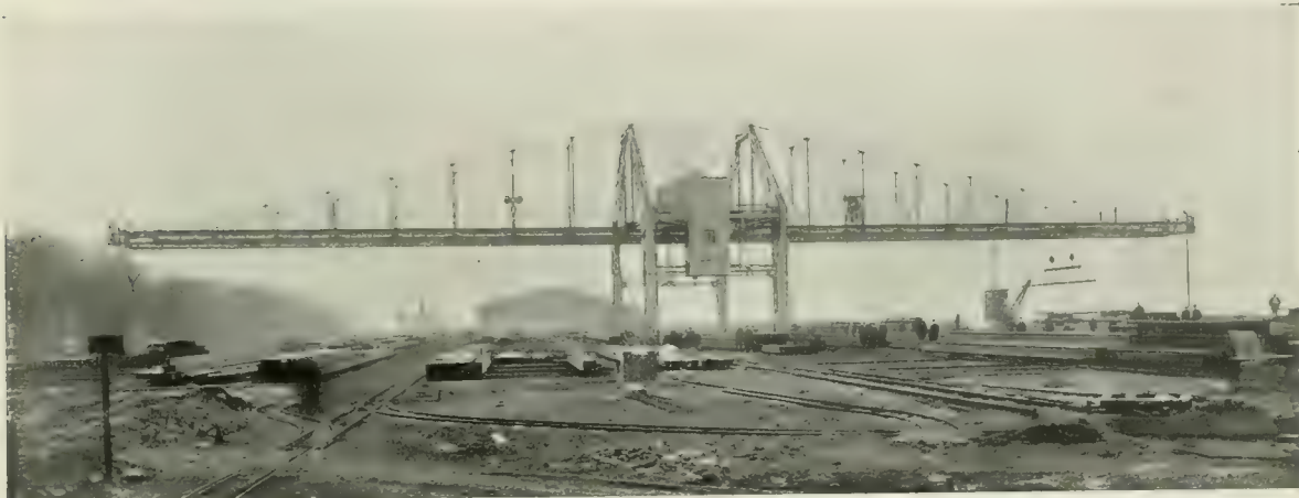
5-ton ELECTRIC TRAVELLING CANTILEVER CRANE. For Stocking and Loading Material. Span : 325 ft.
