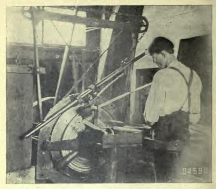
Ffg. 30. Coiling patent barrel hoops made from white elm. Ohio in 1911 leads all other States in the production of this commodity.
