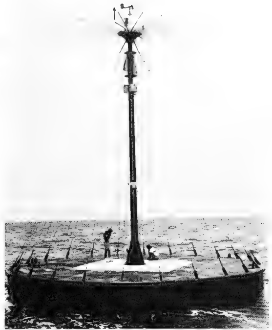
Figure 12. This surface platform is capable of being moored in deep oceans, collects over 100 oceanographic and meteorological parameters, and can transmit them to shore stations 2,500 miles away. (Navy photo)
