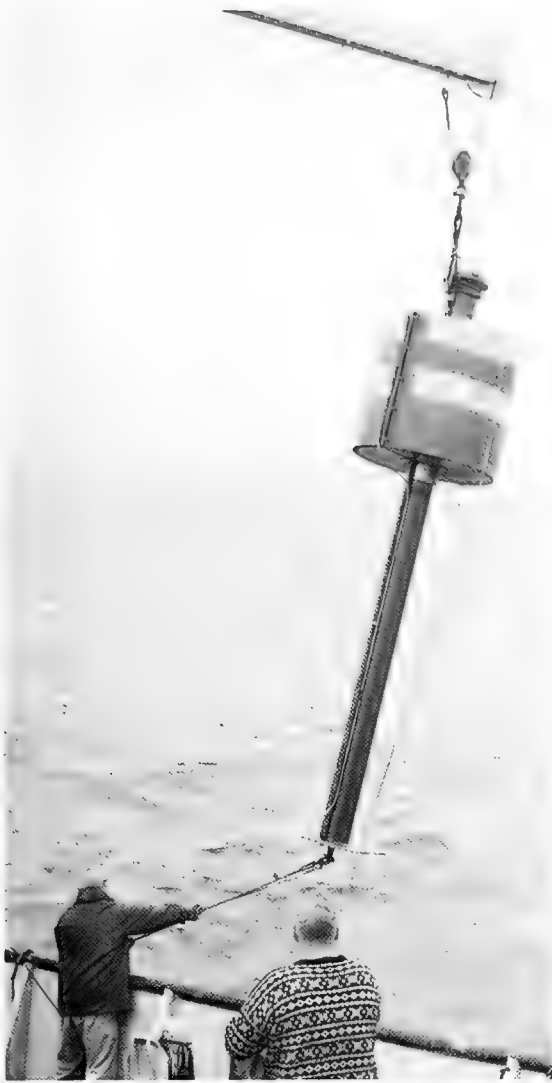
Figure 19. Launching free-drifting buoy with temperature and salinity sensors in the Pacific, as part of BCF program. Data are transmitted to shore station by radio. (Bureau of Commercial Fisheries photo)
