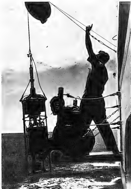
Figure 10. Global scientific expedition 1967. Modern oceanographic observations are utilizing complex electronic instruments such as this salinity-temperature-depth sensor. Although more costly than classical instruments, these instruments portray more accuracy and realistic measurement of the actual ocean structure. (ESSA photo)
