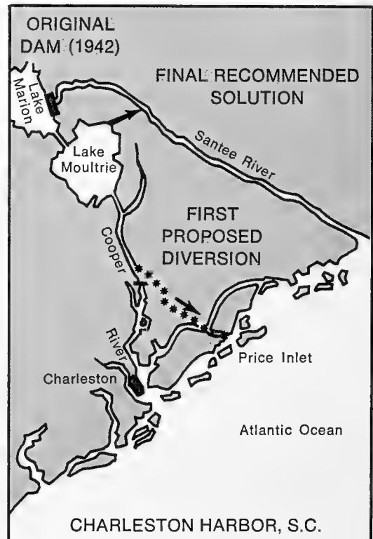
Figure 8. Water diversion: Cooper and Santee Rivers, South Carolina.
