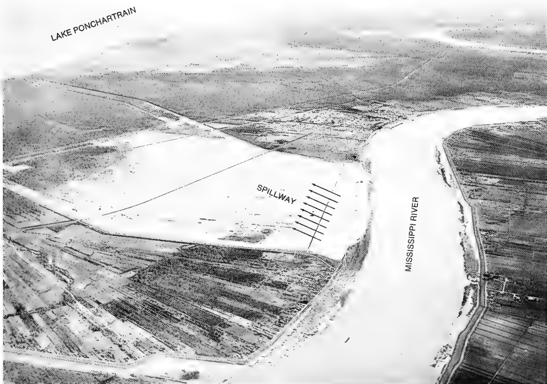
Figure 9. Bonnet Carre Spillway, Louisiana. Mississippi River floodwater is diverted into saltwaters of Lake Pontchartrain. Here flood protection must be weighed against attendant shellfish losses. (U.S. Army Corps of Engineers photo).
