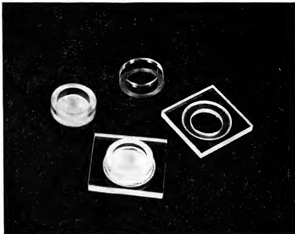
FIG. 1. Components of the culture cells. The one in the lower center is assembled but has no plastic film cover.
