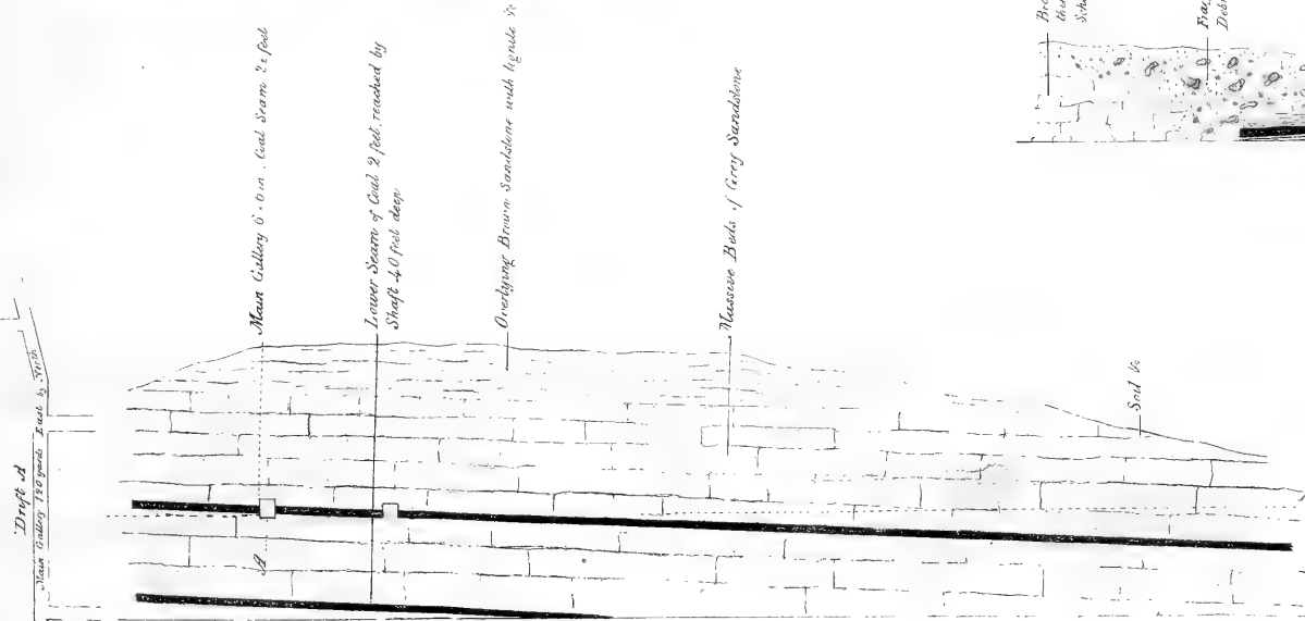
SECTION showing 2 seams of Bituminous Coal each 2 feet thick at Jerusalem.
