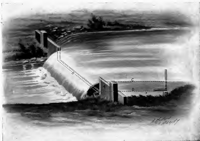
FIG. 9.—Gauging the Discharge of a Stream,
