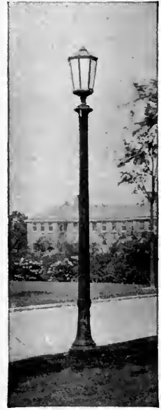
Form 23B Novalux Lantern Unit with Colonial alabaster glass panels and dome refractor, made by the General Electric Company. Union Metal Manufacturing Company pressed steel standard, Design No. 842, 15,000 lumen (1500 c.p.) mazda C lamp. Height to light source, 15 feet.
