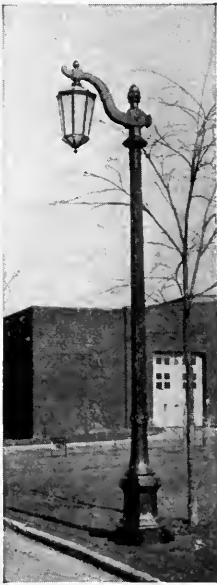
Form 24B Novalux Lantern Unit with Colonial alabaster glass panels and dome refractor, made by the General Electric Company. Union Metal Manufacturing Company pressed steel standard with bracket, Design No. 1106, 10,000 lumen (1000 c.p.) mazda C lamp. Height to light source, 18 feet. Length of bracket arm, 2½ feet.
