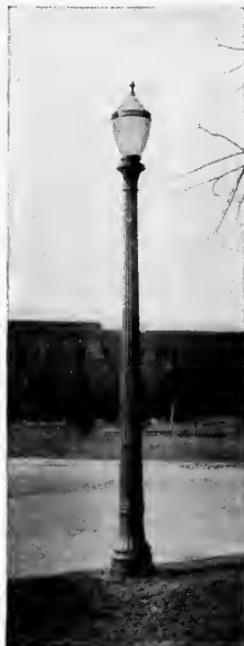
Form 12 Novalux Unit with No. 123 light alabaster rippled glass globe, canopy and dome refractor, made by the General Electric Company. Union Metal Manufacturing Company pressed steel standard, Design No. 1537, 4,000 lumen (400 c.p.) mazda C lamp. Height to light source, 13½ feet.
