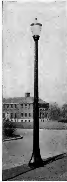
Paragon Senior Top with opalescent rectilinear glass globe, canopy and cast iron post, Design Arcadian A, made by the George Cutter Works of the Westinghouse Electric and Manufacturing Company, 15,000 lumen (1500 c.p.) mazda C lamp. Height to light source, 16 feet.
