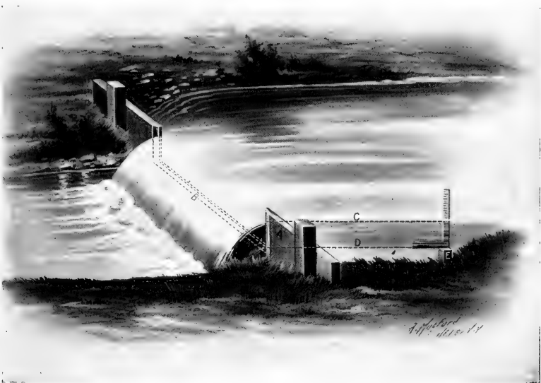
FIG. 9.—Gauging the Discharge of a Stream,
