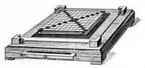
Fig. 84.—Wolfhügel's apparatus for counting colonies of bacteria upon plates.
