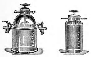
Fig. 63.—Novy's jars for anaerobic cultures.
