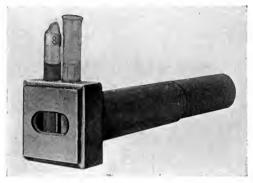
Fig. 92.—The nephelometer; an instrument used for standardizing bacterial suspensions used for the opsonic test or for vaccines, by comparison with precipitate of barium sulphate.
