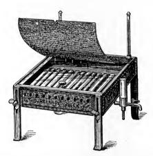
Fig. 46.—Koch's apparatus for coagulating and sterilizing bloodserum.
