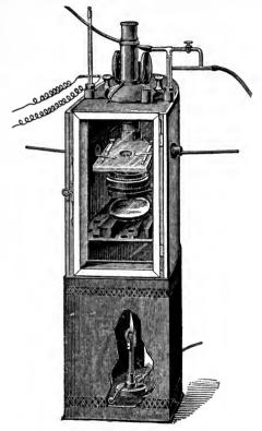
Fig. 33.—Apparatus for keeping objects under microscopic examination at constant temperatures (Nuttall).
