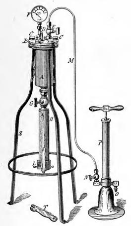
Fig. 41.—Pasteur-Chamberland filter arranged to filter under pressure.
