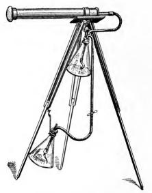
Fig. 81.—Hesse's apparatus for collecting bacteria from the air.
