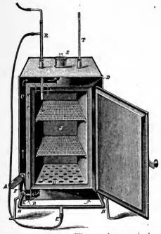
Fig. 38.—Hot-air sterilizer. The gas jets are inclosed within the space between the outer and middle walls, C, and can be seen at F. The heat ascends, warming the air between the two inner walls, which ascends between the walls, K, then descends over the contents, J, and escapes through perforations in the bottom, B, to supply the draft at F, and eventually escapes again at S; R, gas regulator; T, thermometer.
