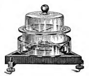
Fig. 52.—Complete leveling apparatus for pouring plate cultures, as taught by Koch.
