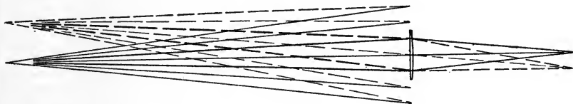
FIG. 2.—Image formation by a single lens. Note that the image, at the right, is \frac{2}{3} the size of the object, in proportion to their respective distances from the lens; the opening angle being \frac{2}{3} the size of the closing angle.
