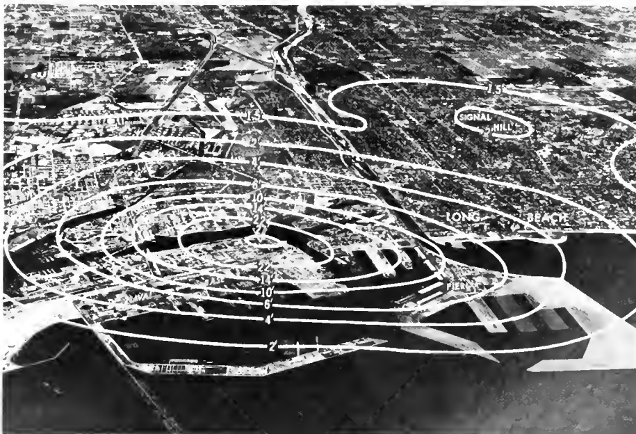
Figure VII-3 — SUBSIDENCE IN LONG BEACH, CALIFORNIA
