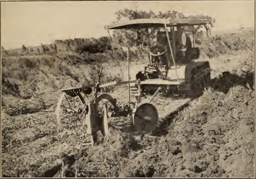
FIG. 1.—SINGLE DISK PLOW WITH SUBSOIL ATTACHMENT. ADAPTED TO PLOWING UNDER PIGEON PEAS FOR GREEN MANURE.
